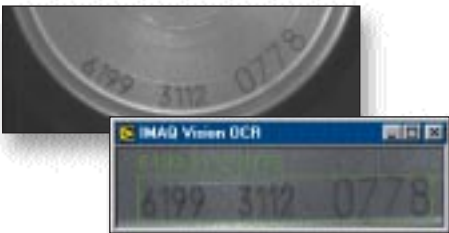
Use IMAQ OCR software to read characters along curves or arcs such as aluminum can lot codes, bottle caps, and CD-ROMs.
