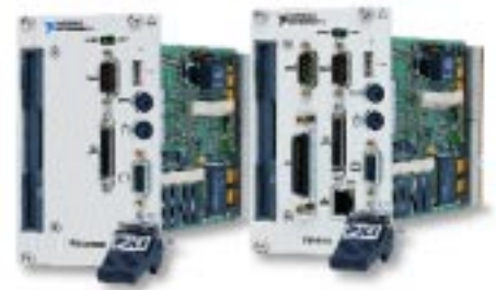
The PXI-8150B Series embedded computers are high-performance system controllers that are compatible with the PXI specification and with CompactPCI.
