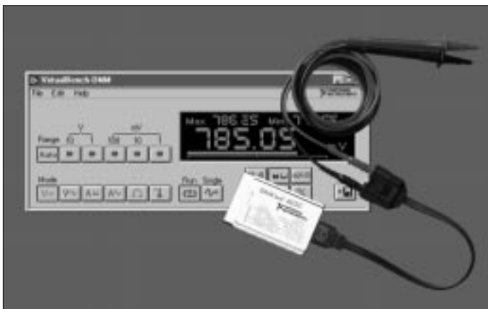
The DAQCard-4050 and VirtualBench-DMM software turn your computer into a digital multimeter.
