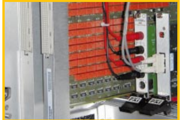
The GR Versa AT combines the GenRad patented PXIscan switching technology with low-cost PXI instruments.
