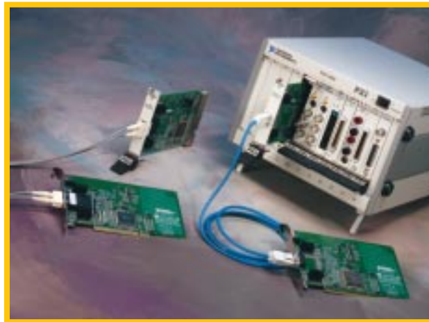
National Instruments MXI-3 is a high-speed serial link for adding more I/O slots to PCs and PXI/CompactPCI systems.
