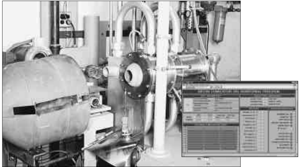
The LabVIEW-monitored 2000° F burner with test samples and top-level VI front panel.
