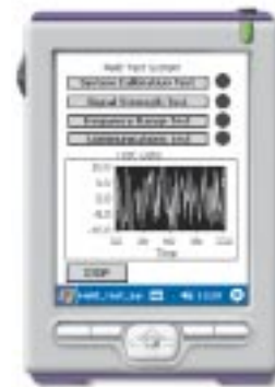
The LabVIEW PDA Module includes an emulator environment for debugging LabVIEW VIs on a PDA when the physical PDA device is unavailable.
