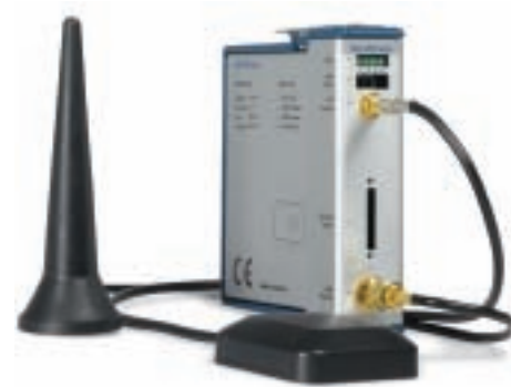
The S.E.A. Gxxx Combo Module includes both wireless GSM and GPS functionality.
