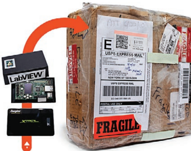
A team of engineers from NI and editors from Popular Mechanics magazine used LabVIEW to measure the acceleration, temperature, and orientation of a package shipped across the United States.
