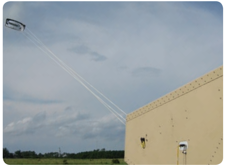
The portable 12 kW airborne wind energy system uses a flexible airfoil to capture power from wind.
