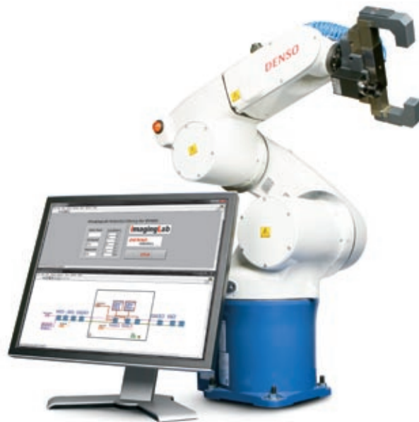
Figure 2. This DENSO robot is controlled with LabVIEW using the ImagingLab Robotics Library for DENSO.
