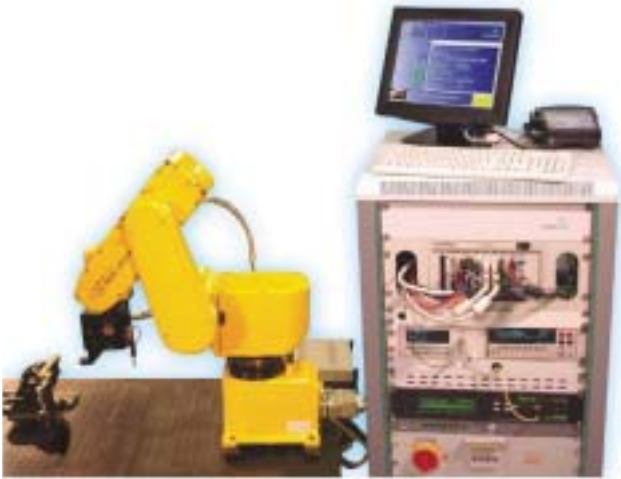
The microassembly system combines robotics and piezo actuators.
