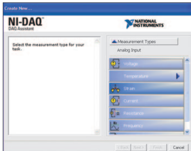
Figure 3. LabVIEW 7 Express DAQ Assistant delivers configuration ease of use and code generation for programming flexibility.
