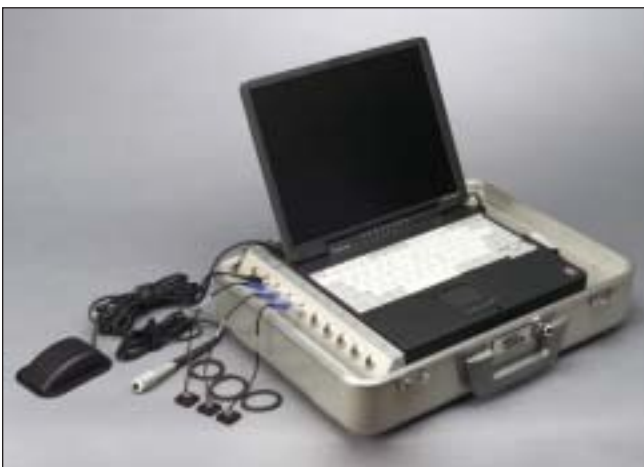
The Ride Quality Analyzer includes a Panasonic Toughbook computer and NI data acquisition hardware for field data acquisition.
