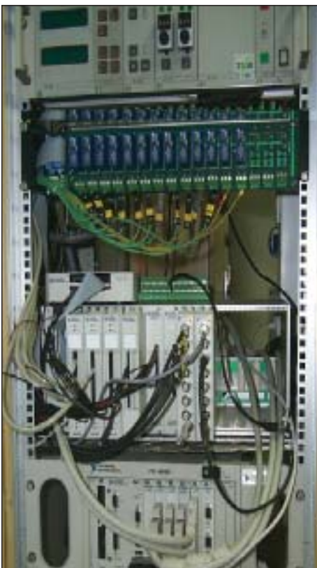
NI PXI and SCXI hardware make it possible to combine multiple signals into one test system.
