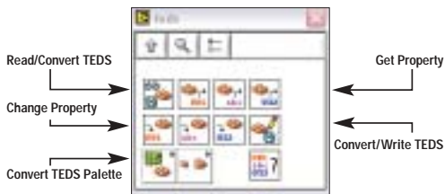
With the TEDS library for LabVIEW 6.1, you can incorporate TEDS into your LabVIEW application.
