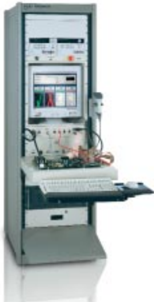
Use the Flextronics Test Model 2598 tester to verify the production test of process control boards.
