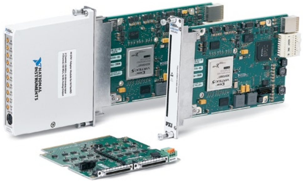
Figure 2. New PXI Express NI FlexRIO FPGA modules interface with I/O adapter modules such as the NI 5781 baseband transceiver.
