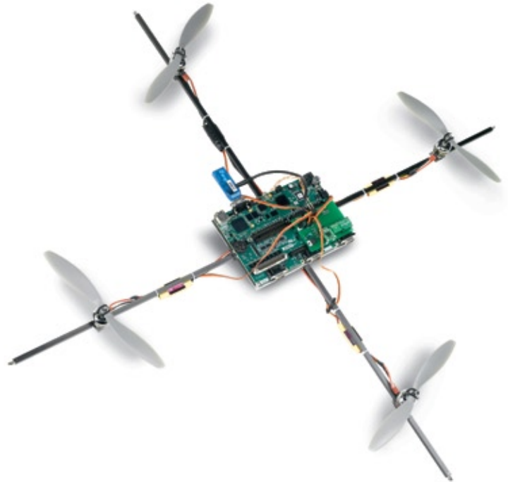
Two NI engineers built a quadrotor helicopter around an NI Single-Board RIO with a control algorithm designed and implemented using the LabVIEW toolchain.
