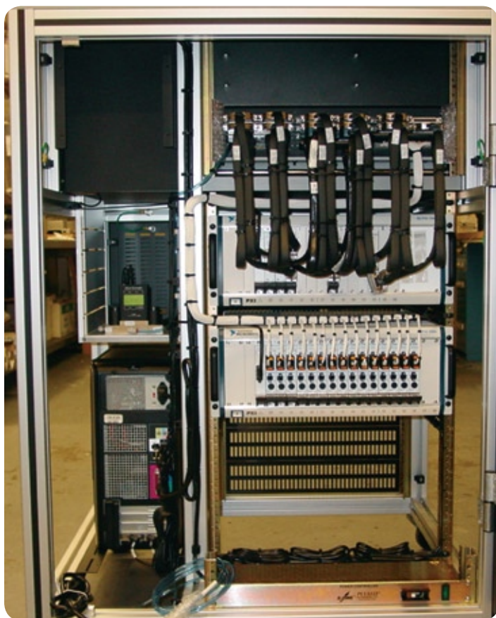
The same FlexATE system, based on NI software and PXI hardware, can test different product designs for increased flexibility.
