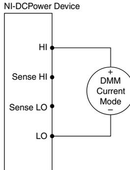
2. Set the **niDCPower Output Function** property or `NIDCPOWER_OUTPUT_FUNCTION` attribute to DC Current for the NI 4141.
