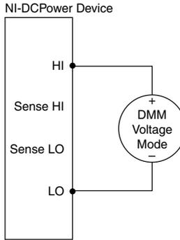
2. Set the **niDCPower Output Function** property or `NIDCPOWER_OUTPUT_FUNCTION` attribute to DC Voltage for the NI 4141.
