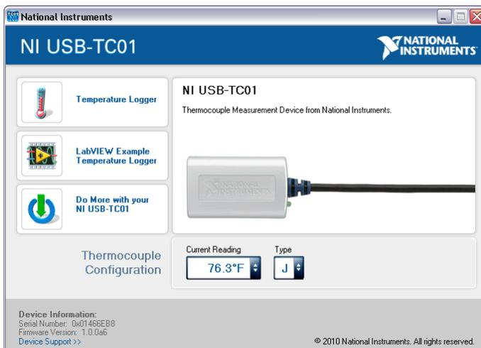
Through the NI USB-TC01 launch screen, you can graph and log data with the Temperature Logger, customize the Temperature Logger source code in LabVIEW, and explore other ways to do more with your NI USB-TC01.
