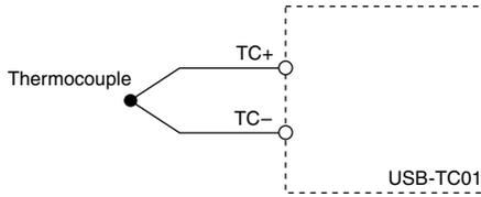
For best results, NI recommends using insulated or ungrounded thermocouples when possible. If you need to increase the length of your thermocouple, use the same type of thermocouple wires to minimize the error introduced by thermal EMFs.
