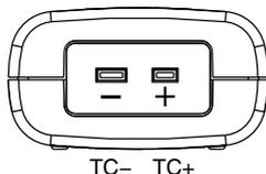
Connect the positive lead of the thermocouple connector to the TC+ terminal, and the negative lead of the thermocouple connector to the TC- terminal.
