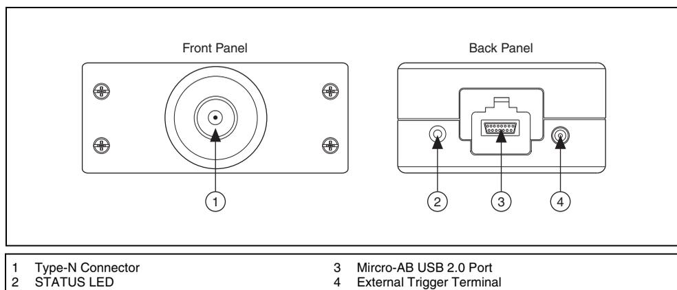
**Figure 4.** NI USB-5681 Front and Back Panel
