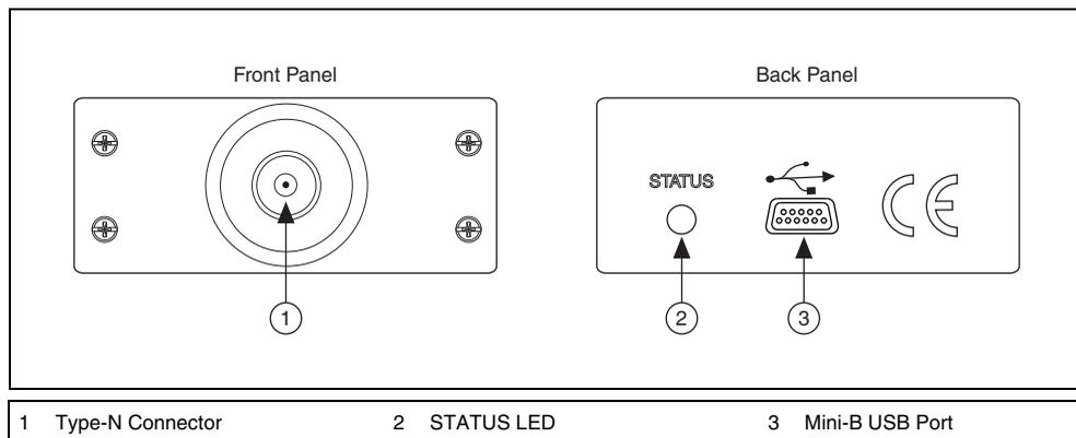
**Figure 3.** NI USB-5680 Front and Back Panel
