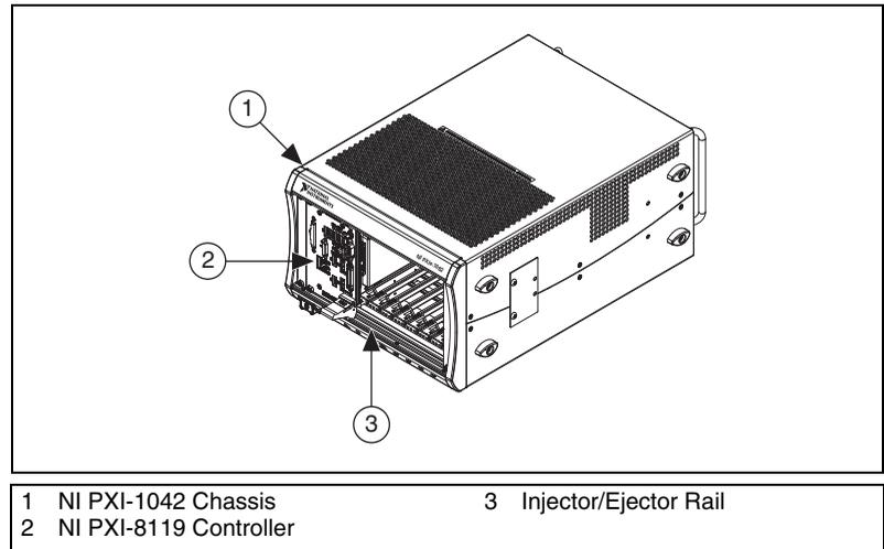
**Figure 2.** NI PXI-8119 Installed in a PXI Chassis
