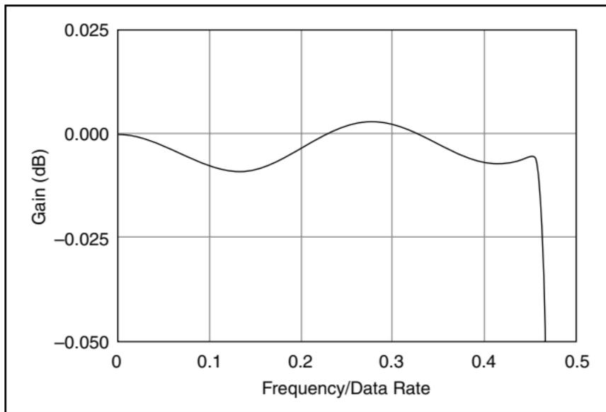
**Figure 6.** Typical Passband Flatness for the NI 9229E/9239E
