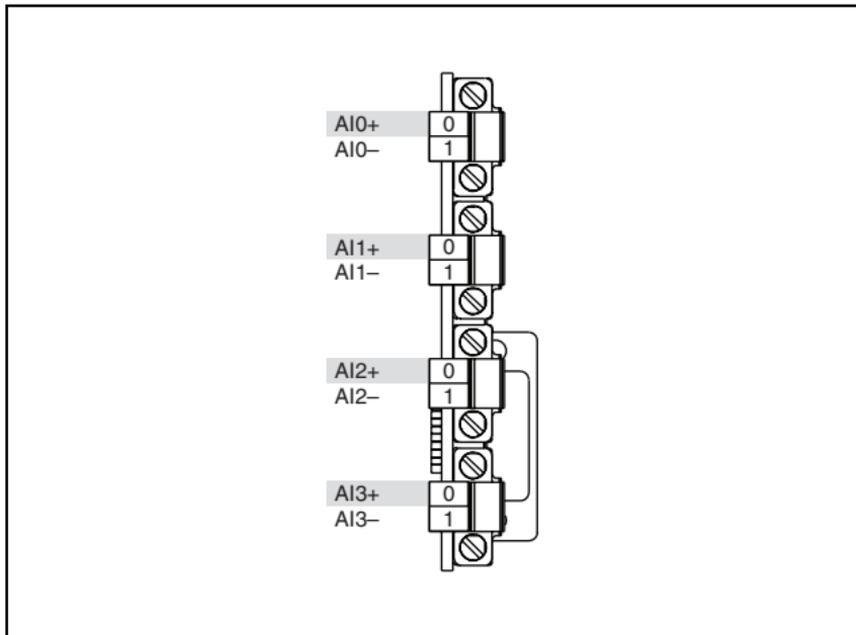
**Figure 2.** NI 9229E/9239E Terminal Assignments
