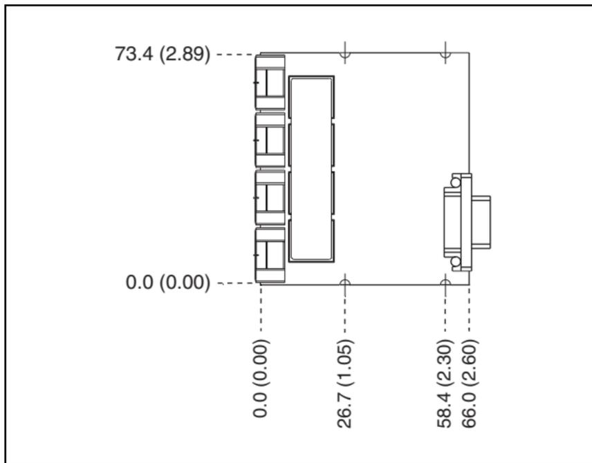
**Figure 1.** NI 9229E/9239E Dimensions in Millimeters (Inches)
