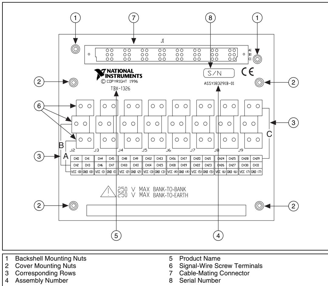
Figure 4. TBX-1326 Parts Locator Diagram
