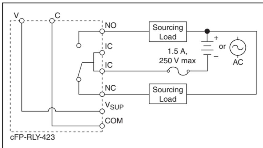
**Figure 2.** Basic Field Connection
