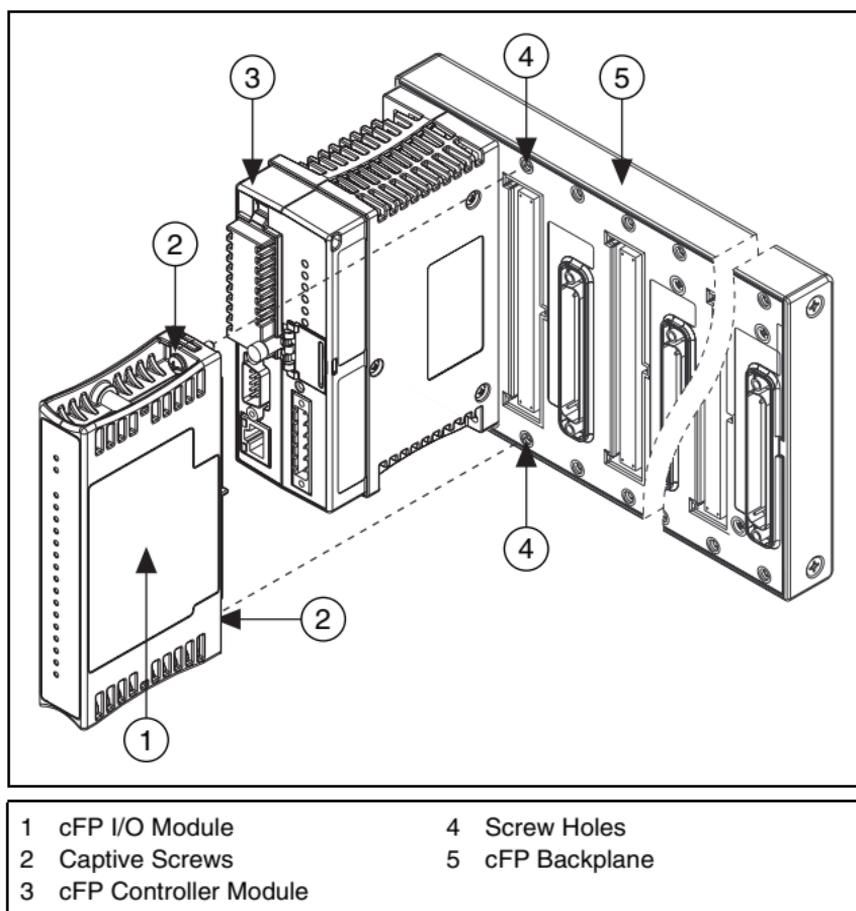
**Figure 1.** Installing the cFP-RLY-423
