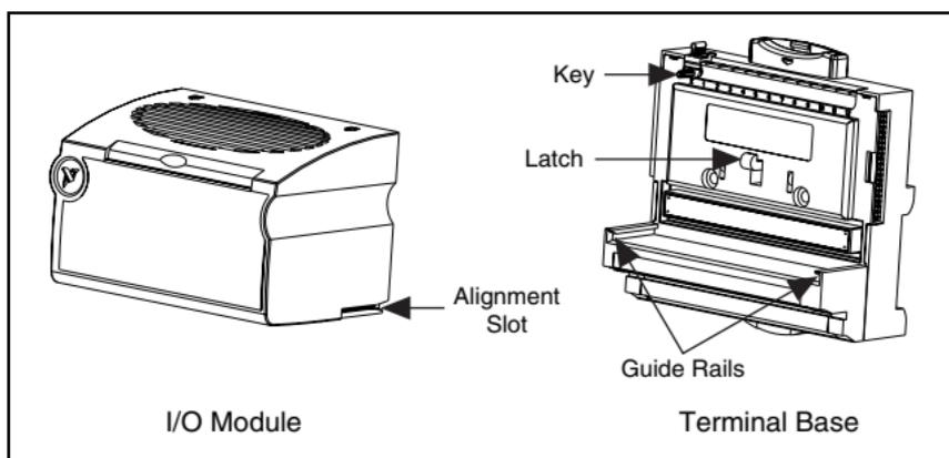
**Figure 1.** Installing the FP-RTD-124
