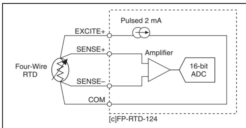
**Figure 3.** FP-RTD-124 Input Circuit
