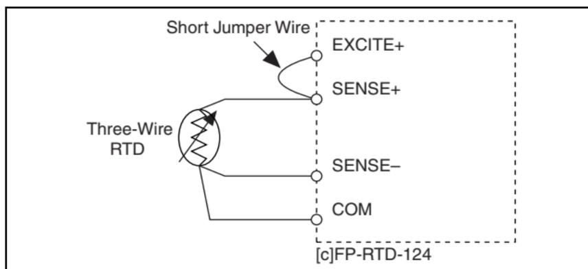
**Figure 5.** Three-Wire RTD Connections on One Channel
