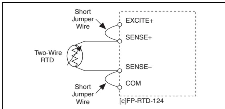
**Figure 6.** Two-Wire RTD Connections on One Channel
