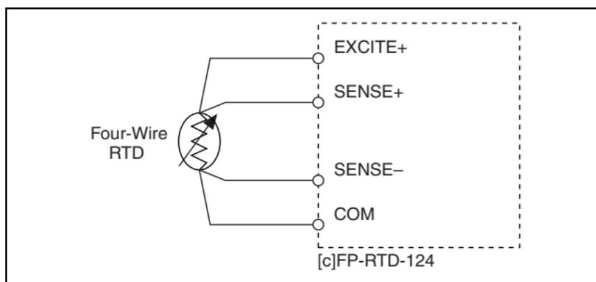
**Figure 4.** Four-Wire RTD Connections on One Channel
