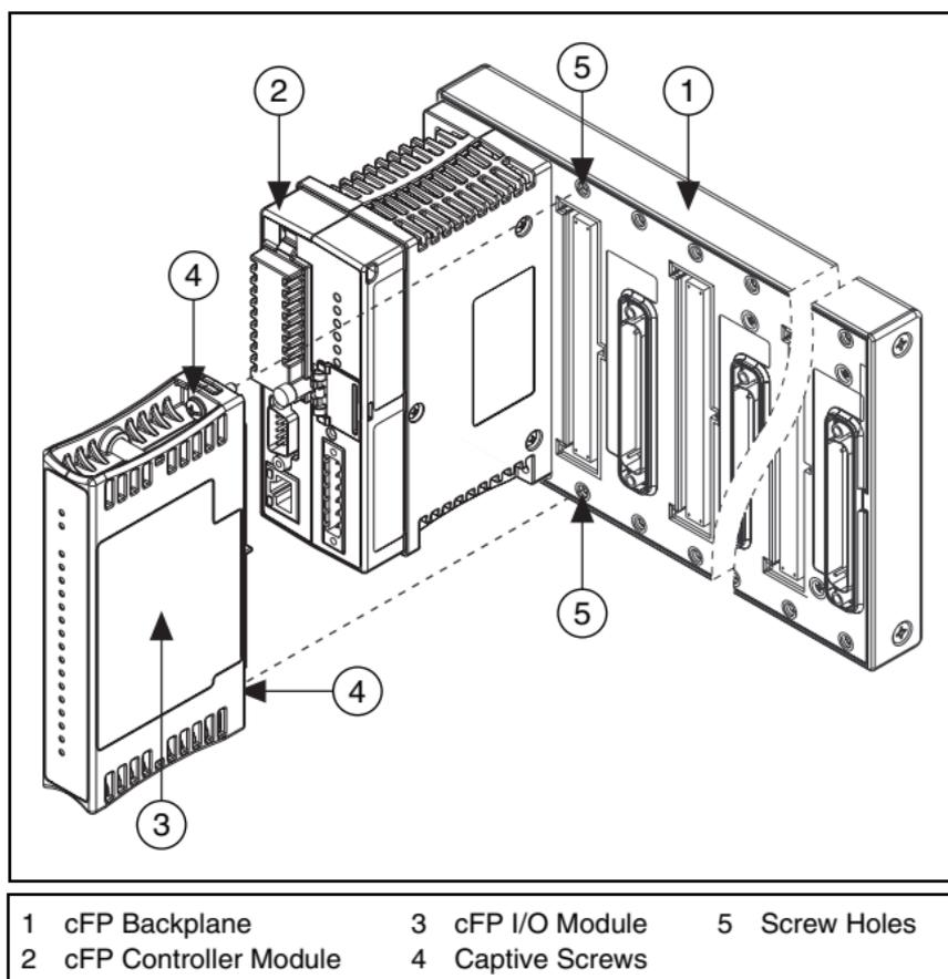
**Figure 2.** Installing the cFP-RTD-124
