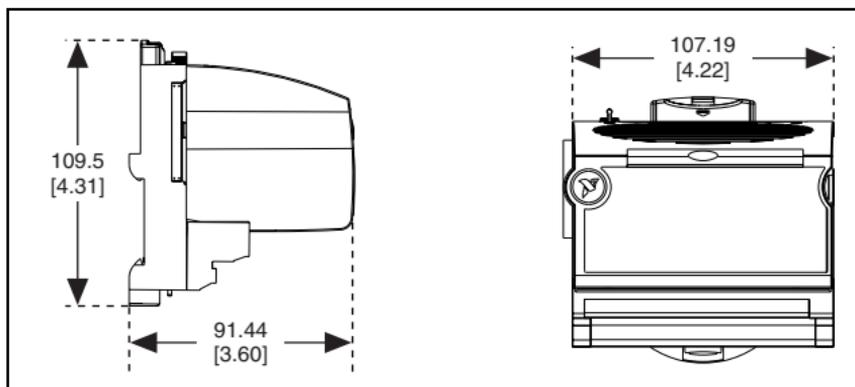
**Figure 7.** FP-RTD-124 Mechanical Dimensions
