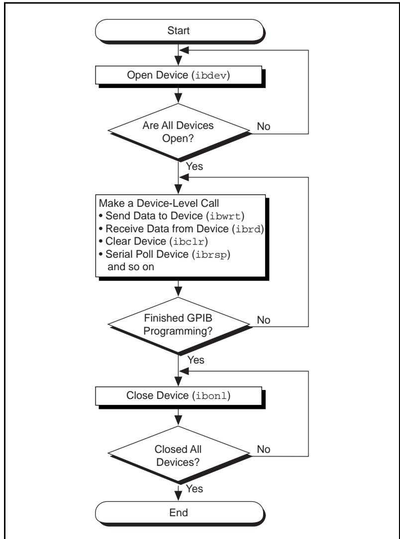
**Figure 2-1.** General Program Shell Using NI-488 Device Functions
