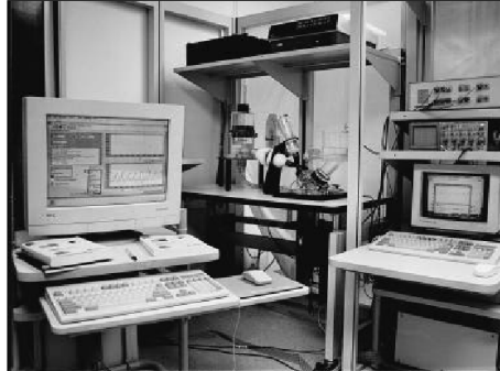
The electromechanical system formed by Structural Acoustics uses Windows-based LabVIEW and DAQ boards on a PC to perform an acoustic diagnostic procedure on prosthetic heart valves.
