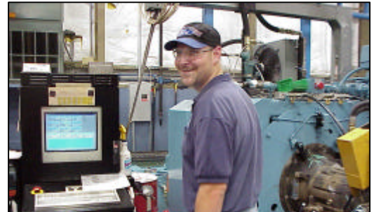
An operator mounts transmissions to be tested, provides input such as manually shifting the unit, and monitors the test status.
