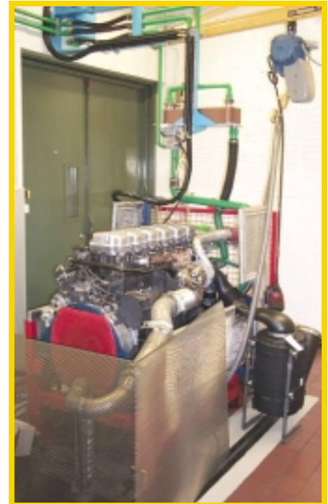
We developed a test system for SCANIA using NI LabVIEW and FieldPoint.
