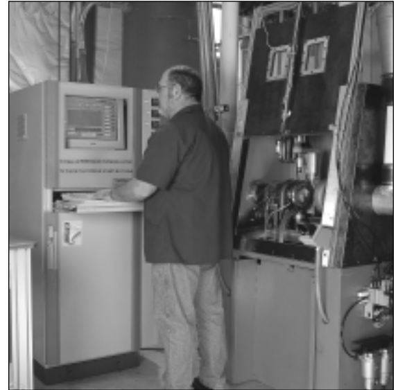
IHI Turbo America Turbo Charger Engine Quality Verification System uses National Instruments LabVIEW RT and hardware.
