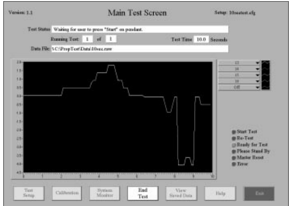
Main User Interface of the Propeller Stress Test System
