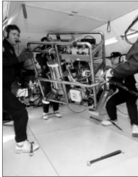
Flight operations personnel from the Reduced Gravity Office at NASA's Lewis Research Center manage the Float Package as it drifts in zero gravity.
