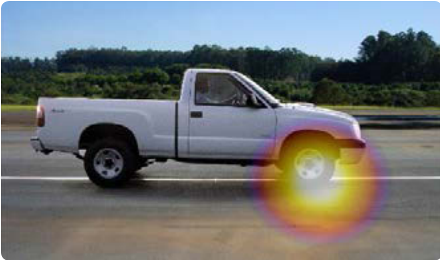
Figure 10. By laying the intensity map from the delay and sum beamforming method over a camera image taken at the same time you recorded the sound, you can visualize the noise source better.
