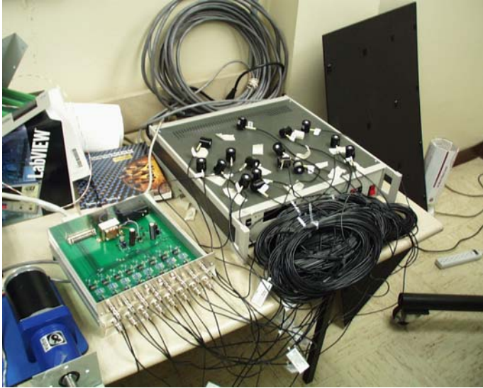
Figure 5. 16-Channel Photo Diode Array located in the Modeling Laboratory.
