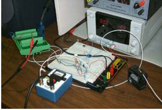
Figure 1: Complete experimental system for motor health monitoring.
