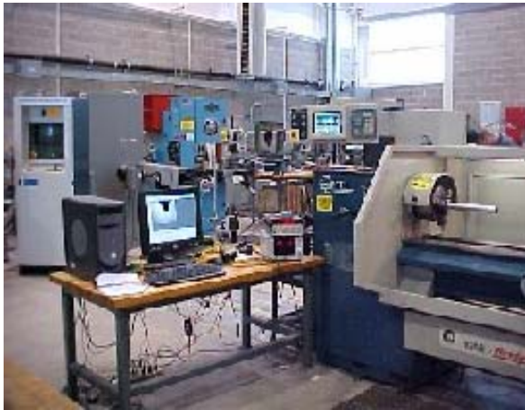
Figure 3: Complete experimental system for AE data collection.
