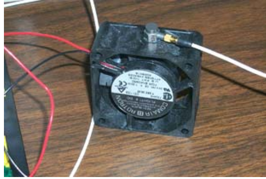
Figure 2: Motor accelerometer set-up.
