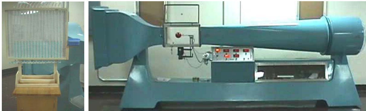
Figure 3. Multi-tube manometer and Aerolab Education Wind Tunnel
