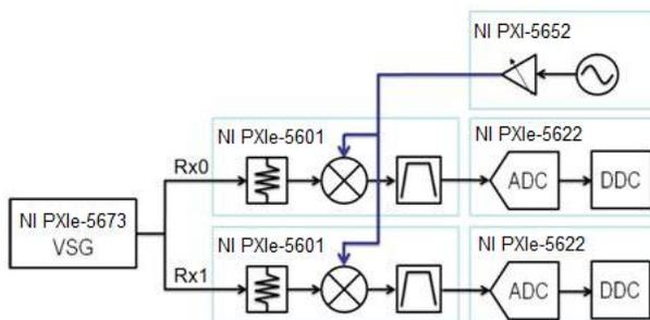
**Figure 7.** Test Setup for Calibrating the Phase of a Two-Channel RF Analyzer
