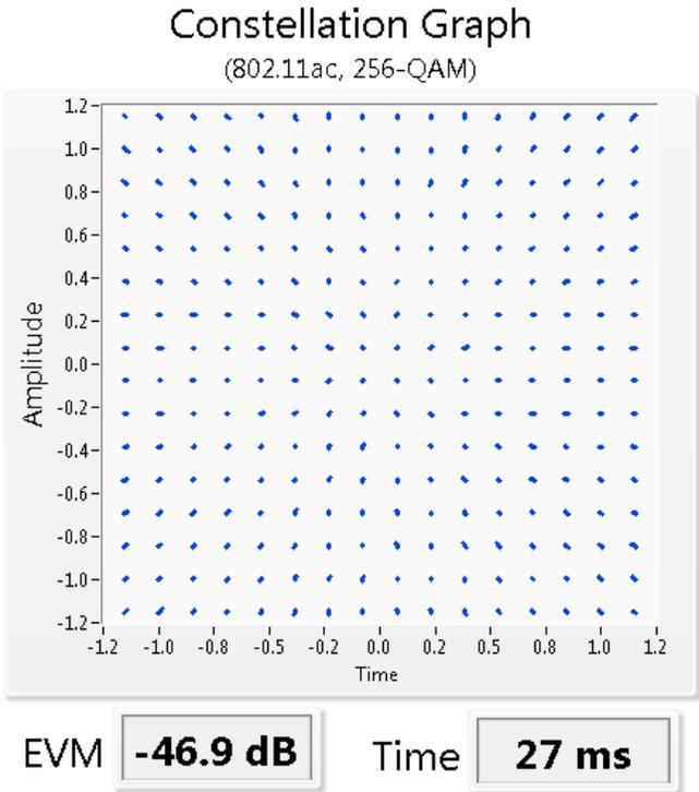
**Figure 2.** Typical Constellation Graph, EVM Measurement, and Measurement Time of an 802.11ac MCS9 Signal at 5.8 GHz.
