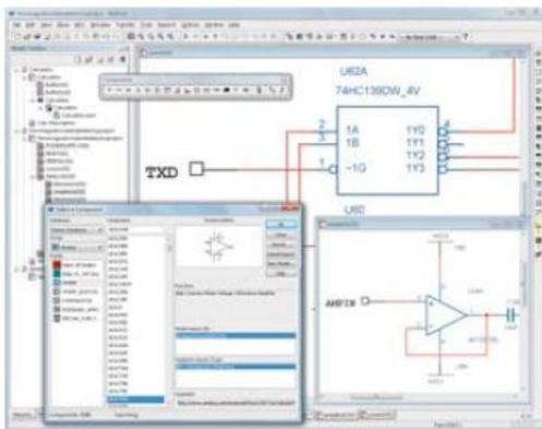
Figure 2. Quickly and easily define circuits in Multisim.
