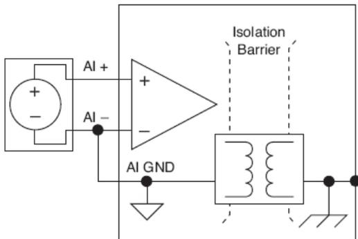
Figure 1. Isolation Barrier on Industrial M Series Devices
