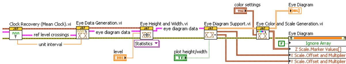
Figure 7. A Typical Workflow for an Eye-Diagram Generation
