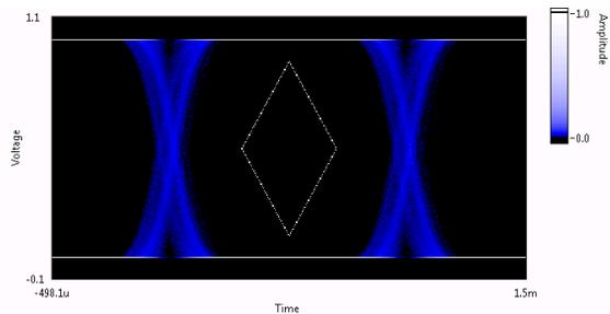
Figure 8. Mask Limit Testing Using a User-Defined Mask
