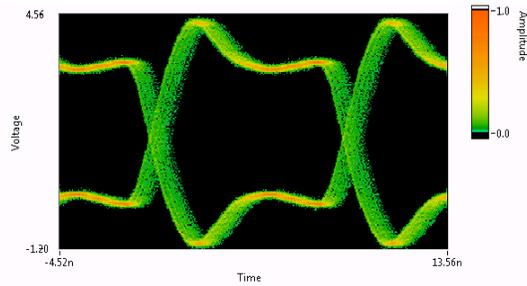
Figure 6. Three-Hue Persistence Eye Diagram
