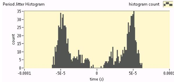
Figure 12. Histogram View of Period Jitter
