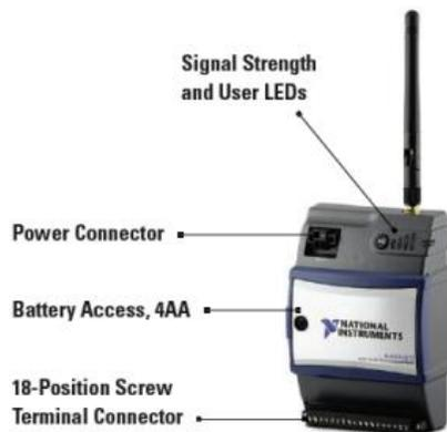
Figure 4. Measurement Node External Features
