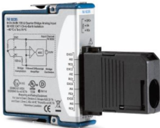
Backshell for NI 9235/9236 Strain Gage Modules
